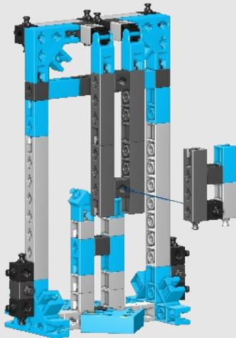
7. For **case 3** switch the additional mass from the neck to the position shown below. In that way you are actually increasing the length of the neck, so that greater velocity is gained just before the collision. Let the neck hit the predator and write your findings on **exercise 3** and **4**.
